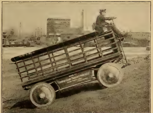
A 4-wheel driven electric wagon on a twenty-five per cent grade, one of the most powerful trucks ever built.
